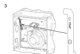
INSTALL HOSE G ON COLLECTOR BOX AS SHOWN. NOTE: LET THE OPEN END HANG FREE UNTIL STEP 10.
