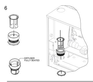
INSTALL INTAKE COUPLING IN BLOWER SHELF HOLE AS SHOWN. INSERT AIR DIFFUSER INTO COUPLING UNTIL RING/TABS ARE SEATED.
