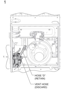
1 - REMOVE CONDENSATE TRAP AND HOSES. (RETAIN HOSE D FOR LATER USE.)
