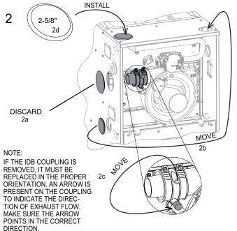
2a-REMOVE 3-3/8" FLUSH MOUNT PLUG FROM JACKET - DISCARD. 2b-RELOCATE 2-3/8" FLUSH MOUNT PLUG FROM JACKET TO TOP PLATE. 2c-RELOCATE 1/2" VINYL CAP (YELLOW) IN INDUCER COUPLING. 2d-INSTALL 2-5/8" FLUSH PLUG IN TOP PLATE.
