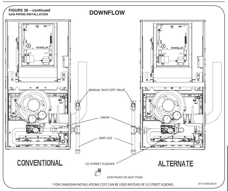
**IMPORTANT:** When making gas pipe connections, use a back-up wrench to prevent any twisting of the main gas valve and manifold. Do not overtighten gas valve on pipe.
