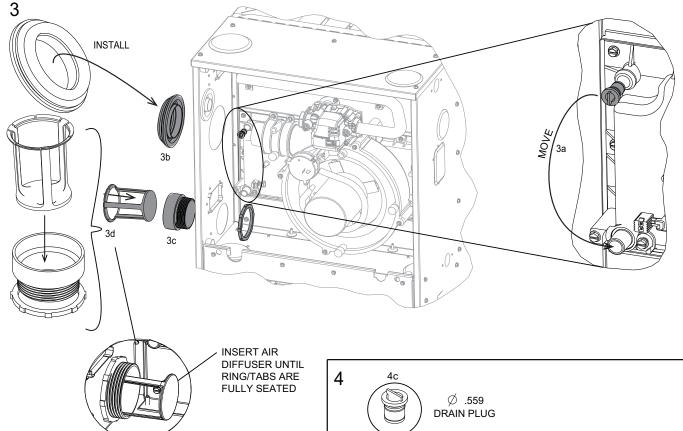
NOTE: DIFFUSER MAY HAVE A TENDENCEY TO FALL OUT OF THE COUPLING AT THIS STEP. THE INSTALLER MAY ELECT TO INSTALL THE DIFFUSER AFTER ROTATING THE FURNACE TO THE HORIZONTAL POSITION.
