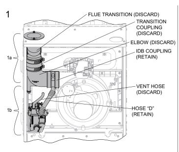
1a - REMOVE FLUE TRANSITION, TRANSITION COUPLING, AND ELBOW. (NOTE: REMOVE COUPLING ON INDUCER WITH ELBOW FOR EASIER REMOVAL).
