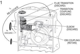
1a - REMOVE FLUE TRANSITION, TRANSITION COUPLING, AND ELBOW.
