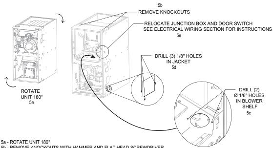
5b - REMOVE KNOCKOUTS WITH HAMMER AND FLAT HEAD SCREWDRIVER.
