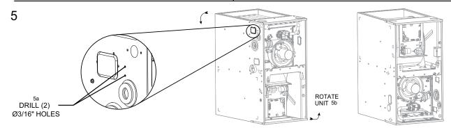
5a - PRE-DRILL (2) Ø 3/16" HOLES IN JACKET AS SHOWN FOR CONDENSATE TRAP BRACKET.
