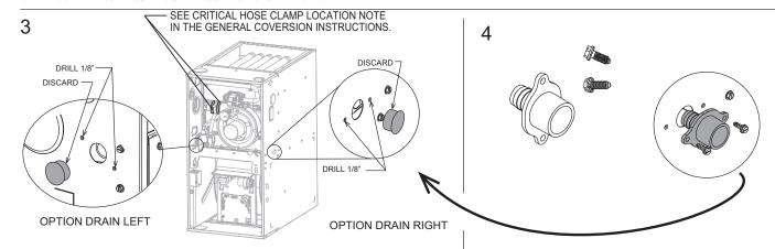
DETERMINE RIGHT OR LEFT DRAIN OPTION. LOCATE 7/8" HOLE IN JACKET SIDE. REMOVE PLUG - DISCARD DRILL (2) ø1/8" HOLES FOR THE BULKHEAD COUPLING. INSTALL BULKHEAD COUPLING USING (2) SCREWS. INSTALL IN JACKET WITH THE BARBED FITTING POINTED INTO THE VESTIBULE.
