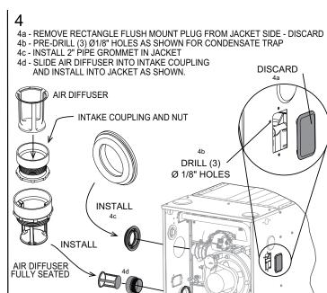
NOTE: DIFFUSER MAY HAVE A TENDENCEY TO FALL OUT OF THE COUPLING AT THIS STEP. THE INSTALLER MAY ELECT TO INSTALL THE DIFFUSER AFTER ROTATING THE FURNACE TO THE HORIZONTAL POSITION.
