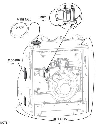
IF THE IDB COUPLING IS REMOVED, IT MUST BE REPLACED IN THE PROPER ORIENTATION. AN ARROW IS PRESENT ON THE COUPLING TO INDICATE THE DIRECTION OF EXHAUST FLOW. MAKE SURE THE ARROW POINTS IN THE CORRECT DIRECTION.
