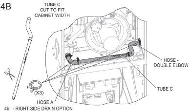
4b1 - CUT TUBE "C" TO FIT CORRESPONDING CABINET WIDTH.
