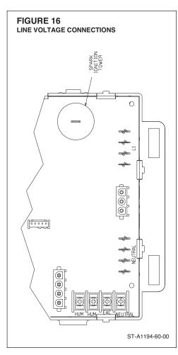
**NOTE:** Do not use 24 volt control wiring smaller than No. 18 AWG.
