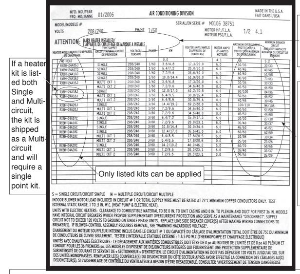
Contractor should "mark or check" the left column for the kit installed.
