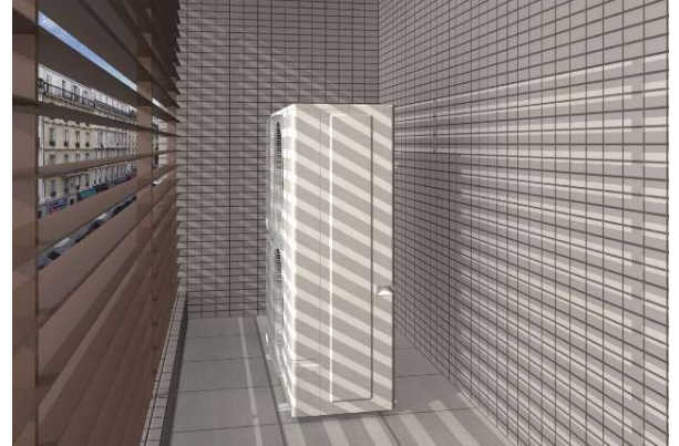
An example of an outdoor unit placed behind a block-out fence on the balcony (conceptual drawing)
