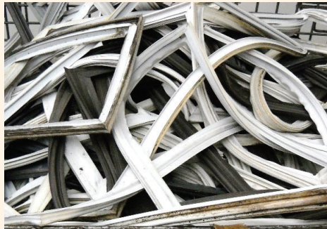
Door packing recovered from refrigerator door
