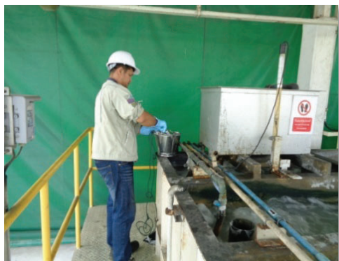
Collecting water quality sample from wastewater treatment system at FGA (THAILAND) CO., LTD.
