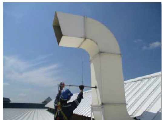
Collection of air quality sample of exhaust duct at FGA (THAILAND) CO., LTD.
