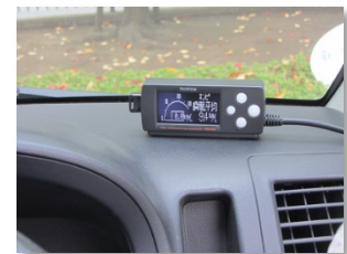
Fuel meter installed
