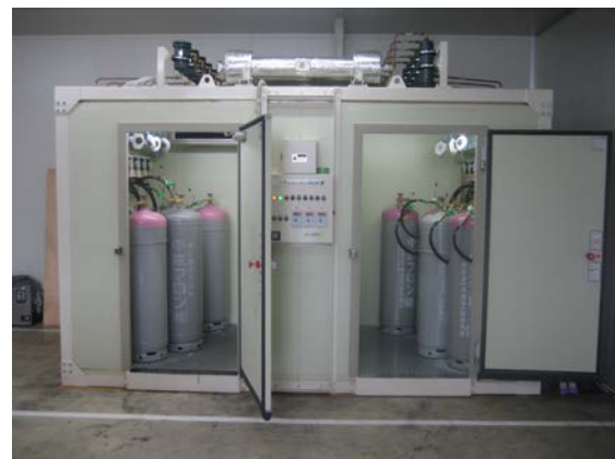
Fluorocarbons regeneration device in Hamamatsu Business Office
