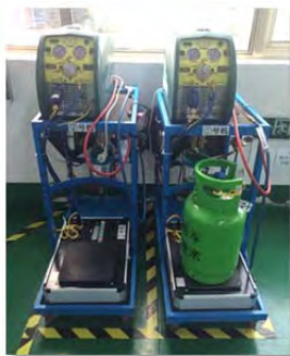
Refrigerant collection equipment of Fujitsu General (Shanghai)
